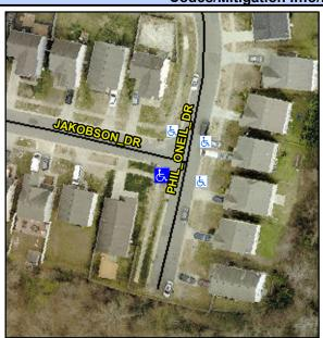
PHIL ONEIL DR Street 1 Name Stop Condition-Street 2 Street 2 Name **JAKOBSON DR** Stop Condition-Street 1 StopSign Possible Solutions: Remove & Replace Curb Ramp With **Two New Directional Ramps or** Equivalent. Surveyor Notes: N/A PROW/ADA: Not Found, R304.5.3
