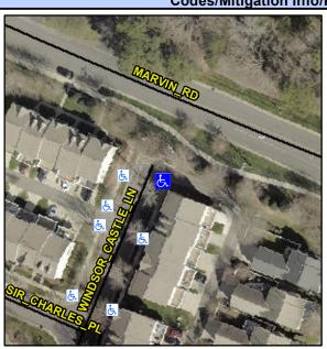
N/A Street 1 Name Stop Condition-Street 2 None WINDSOR CASTLE LN Street 2 Name Stop Condition-Street 1 None Possible Solutions: Remove & Replace Curb Ramp With Two New Directional Ramps or Equivalent. Surveyor Notes: N/A PROW/ADA:
