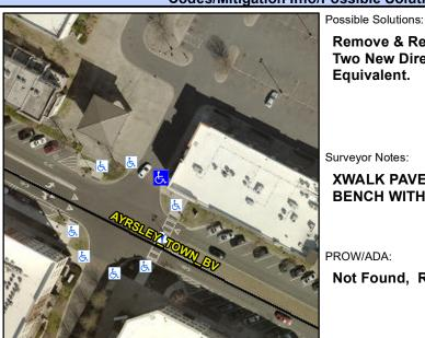
**ENTRANCE** Street 1 Name Stop Condition-Street 1 StopSign Street 2 Name N/A Stop Condition-Street 2 N/A Remove & Replace Curb Ramp With Two New Directional Ramps or Equivalent.
