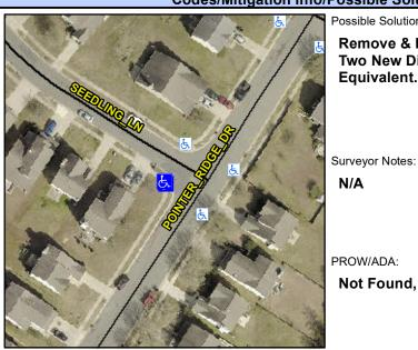
Street 1 Name Stop Condition-Street 2 Street 2 Name Stop Condition-Street 1 POINTER RIDGE DR None **SEEDLING LN** StopSign Possible Solutions: Remove & Replace Curb Ramp With **Two New Directional Ramps or** Equivalent.
