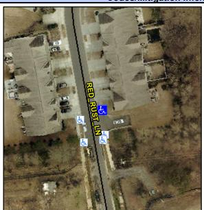
**RED RUST LN** Street 1 Name Stop Condition-Street 2 None Street 2 Name N/A Stop Condition-Street 1 None Possible Solutions: Remove & Replace Curb Ramp With **Two New Directional Ramps or** Equivalent. Surveyor Notes: N/A PROW/ADA: Not Found, R304.2.2, R304.5.3
