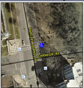
**BARCLAY DOWNS DR** Street 1 Name Stop Condition-Street 2 Signal **CARNEIGIE BV** Street 2 Name Stop Condition-Street 1 Signal Possible Solutions: Remove & Replace Curb Ramp With Two New Directional Ramps or Equivalent. Surveyor Notes: N/A PROW/ADA: Not Found, R304.2.2, R304.5.3
