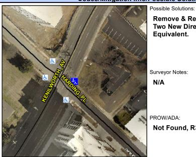
**KENILWORTH AV** Street 1 Name Stop Condition-Street 2 Street 2 Name HARDING PL Stop Condition-Street 1 StopSign Remove & Replace Curb Ramp With Two New Directional Ramps or Equivalent.
