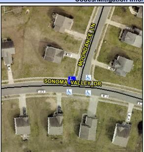
Street 1 Name Stop Condition-Street 2 Street 2 Name Stop Condition-Street 1 **SONOMA VALLEY DR** None **MOONDANCE LN** StopSign Possible Solutions: **Remove & Replace Curb Ramp With Two New Directional Ramps or** Equivalent. Surveyor Notes: N/A PROW/ADA: Not Found, R304.5.1
