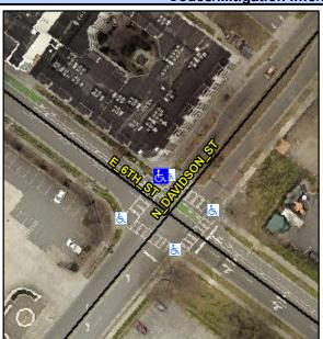
E 6TH ST Street 1 Name Stop Condition-Street 2 Signal Street 2 Name N/A Stop Condition-Street 1 N/A Possible Solutions: Remove & Replace Entire Ramp. Surveyor Notes: N/A PROW/ADA: Not Found, R304.5.1, R304.2.2, R304.5.3
