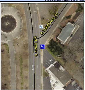
Street 1 Name Stop Condition-Street 2 Street 2 Name Stop Condition-Street 1 S TORRENCE ST StopSign **S KINGS DR** None Possible Solutions: Remove & Replace Curb Ramp With **Two New Directional Ramps or** Equivalent. Surveyor Notes: N/A PROW/ADA: R304.2.2, R304.5.3
