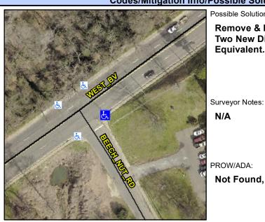
Street 1 Name Stop Condition-Street 2 Street 2 Name Stop Condition-Street 1 **WEST BV** None Possible Solutions: Remove & Replace Curb Ramp With Two New Directional Ramps or Equivalent.
