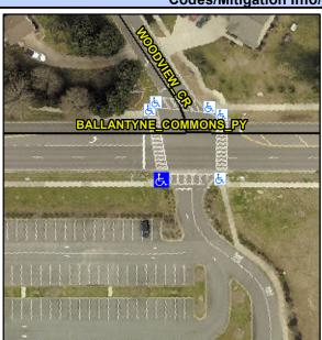
**ENTRANCE** Street 1 Name Stop Condition-Street 2 Signal **BALLANTYNE COMMONS PY** Street 2 Name Stop Condition-Street 1 Signal Remove & Replace Curb Ramp With Two New Directional Ramps or Equivalent.
