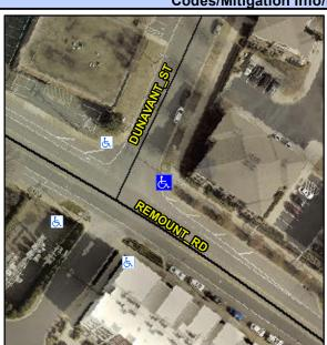
Street 1 Name Stop Condition-Street 2 Street 2 Name Stop Condition-Street 1 **DUNAVANT ST** StopSign **REMOUNT RD** None Possible Solutions: Remove & Replace Curb Ramp With Two New Directional Ramps or Equivalent. Surveyor Notes: N/A PROW/ADA: Not Found, R304.2.2
