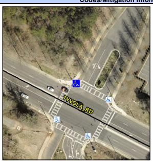
Street 1 Name None Stop Condition-Street 1 **TYVOLA RD** Street 2 Name StopSign Stop Condition-Street 2 N/A Possible Solutions: Remove & Replace Curb Ramp With Two New Directional Ramps or Equivalent. Surveyor Notes: **MEDIAN ACROSS TYVOLA RD** PROW/ADA
