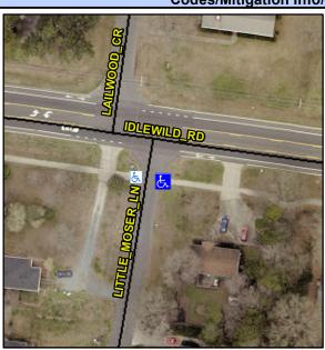
LITTLE MOSER LN Street 1 Name Stop Condition-Street 1 StopSign N/A Street 2 Name Stop Condition-Street 2 N/A Possible Solutions: Compliance Description N/A Remove & Replace Curb Ramp With Two New Directional Ramps or Yes Equivalent. N/A N/A N/A N/A Surveyor Notes: N/A **NO CURB LINE** N/A N/A N/A N/A PROW/ADA: N/A R304.5.3 N/A N/A
