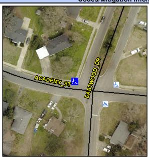
**EASTWOOD DR** Street 1 Name Stop Condition-Street 1 StopSign N/A Street 2 Name Stop Condition-Street 2 N/A Remove & Replace Curb Ramp With Two New Directional Ramps or Equivalent.
