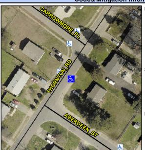
THORNTON RD Street 1 Name Stop Condition-Street 2 None Street 2 Name N/A Stop Condition-Street 1 N/A Possible Solutions: Remove & Replace Entire Ramp. Surveyor Notes: N/A PROW/ADA: Not Found, R304.2.1, R304.2.2-Perp, R304.3.2-Para, R304.5.3
