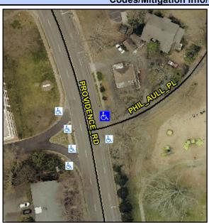
Street 1 Name Stop Condition-Street 2 Street 2 Name Stop Condition-Street 1 **PROVIDENCE RD** None **PHIL AULL PL** StopSign Possible Solutions: Remove & Replace Curb Ramp With **Two New Directional Ramps or** Equivalent. Surveyor Notes: N/A PROW/ADA: Not Found, R304.2.2, R304.5.3
