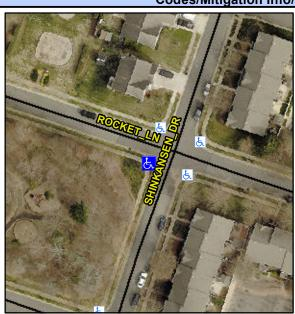
Street 1 Name Stop Condition-Street 2 Street 2 Name Stop Condition-Street 1 SHINKANSEN DR None **ROCKET LN** StopSign Possible Solutions: Remove & Replace Curb Ramp With **Two New Directional Ramps or** Equivalent. Surveyor Notes: N/A PROW/ADA: Not Found, R304.5.3
