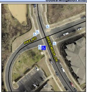
**BRENTMOOR DR** Street 1 Name Stop Condition-Street 2 None **PIKE RD** Street 2 Name Stop Condition-Street 1 StopSign Possible Solutions: Remove & Replace Curb Ramp With Two New Directional Ramps or Equivalent. Surveyor Notes: N/A PROW/ADA: Not Found, R304.5.1
