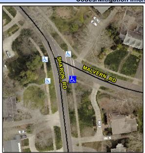
**MALVERN RD** Street 1 Name Stop Condition-Street 2 StopSign **SHARON RD** Street 2 Name Stop Condition-Street 1 None Possible Solutions: Compliance Description N/A Remove & Replace Curb Ramp With Two New Directional Ramps or No Equivalent. N/A Surveyor Notes: N/A PROW/ADA: R304.5.1, R304.2.2, R304.5.3
