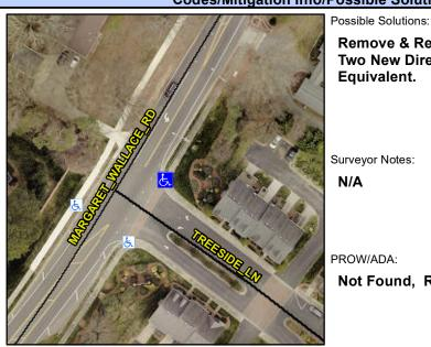
**MARGARET WALLACE RD** Street 1 Name Stop Condition-Street 1 Street 2 Name TREESIDE LN Stop Condition-Street 2 StopSign Remove & Replace Curb Ramp With Two New Directional Ramps or Equivalent.
