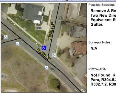
**LOUISE AV** Street 1 Name Stop Condition-Street 1 StopSign Street 2 Name N/A Stop Condition-Street 2 N/A Remove & Replace Curb Ramp With Two New Directional Ramps or Equivalent. Remove & Replace Gutter.
