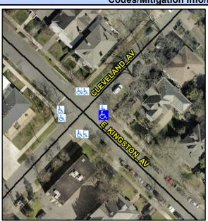
**E KINGSTON AV** Street 1 Name Stop Condition-Street 1 StopSign N/A Street 2 Name Stop Condition-Street 2 N/A Possible Solutions: Remove & Replace Entire Ramp. Surveyor Notes: **NO CURB LINE, ASP LIP 1.0"** PROW/ADA: R304.2.2, R304.5.3
