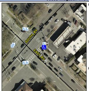
Street 1 Name **EAST BV** Stop Condition-Street 1 Signal Street 2 Name N/A Stop Condition-Street 2 N/A Remove & Replace Curb Ramp With Two New Directional Ramps or Equivalent.
