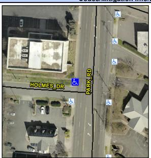
**HOLMES DR** Street 1 Name Stop Condition-Street 1 StopSign Street 2 Name N/A Stop Condition-Street 2 N/A Possible Solutions: **Remove & Replace Curb Ramp With** Two New Directional Ramps or Equivalent. Surveyor Notes: N/A PROW/ADA: R304.5.3
