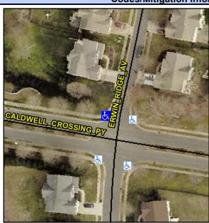
Street 1 Name **CALDWELL CROSSING PY** Stop Condition-Street 2 None **ERWIN RIDGE AV** Street 2 Name Stop Condition-Street 1 StopSign Possible Solutions: Compliance Description N/A Remove & Replace Curb Ramp With Two New Directional Ramps or No Equivalent. N/A N/A N/A N/A Surveyor Notes: N/A N/A N/A N/A N/A N/A PROW/ADA: N/A Not Found, R304.5.1 N/A N/A N/A
