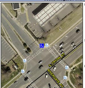
**RIVERGATE PY** Street 1 Name Stop Condition-Street 2 Signal Street 2 Name N/A Stop Condition-Street 1 N/A Possible Solutions: Remove & Replace Entire Ramp. Surveyor Notes: N/A PROW/ADA: Not Found, R304.5.3, R304.2.1, R304.2.2-Perp, R304.3.2-Para, R305.2
