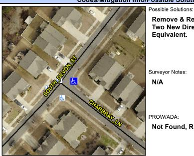
Street 1 Name Stop Condition-Street 2 Street 2 Name Stop Condition-Street 1 **SOUTH DEVON ST** None **CHARBRAY LN** StopSign **Remove & Replace Curb Ramp With Two New Directional Ramps or** Equivalent.
