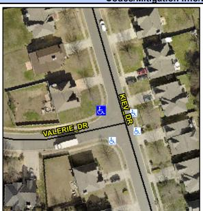
**VALERIE DR** Street 1 Name Stop Condition-Street 2 StopSign **KIEV DR** Street 2 Name Stop Condition-Street 1 None Possible Solutions: Remove & Replace Curb Ramp With Two New Directional Ramps or Equivalent. Surveyor Notes: N/A
