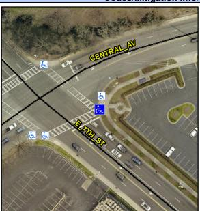
Street 1 Name Stop Condition-Street 1 Street 2 Name Stop Condition-Street 2 Remove & Replace Curb Ramp With Two New Directional Ramps or Equivalent.
