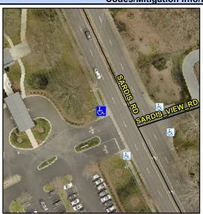
**ENTRANCE** Street 1 Name Stop Condition-Street 2 None Street 2 Name **SARDIS RD** Stop Condition-Street 1 None Possible Solutions: Remove & Replace Curb Ramp With **Two New Directional Ramps or** Equivalent. Surveyor Notes: N/A PROW/ADA: Not Found, R304.5.1, R304.5.3
