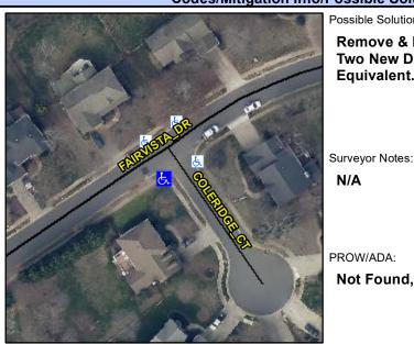
Street 1 Name Stop Condition-Street 2 Street 2 Name Stop Condition-Street 1 **COLERIDGE CT** StopSign **FAIRVISTA DR** None Possible Solutions: Remove & Replace Curb Ramp With Two New Directional Ramps or Equivalent.
