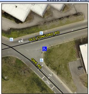
OLD CONCORD RD Street 1 Name Stop Condition-Street 2 None Street 2 Name N/A Stop Condition-Street 1 N/A Possible Solutions: Remove & Replace Entire Ramp. Surveyor Notes: N/A PROW/ADA: Not Found, R304.2.2, R304.5.3
