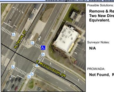
N TRYON ST Street 1 Name Stop Condition-Street 1 Signal Street 2 Name N/A Stop Condition-Street 2 N/A Remove & Replace Curb Ramp With Two New Directional Ramps or Equivalent.
