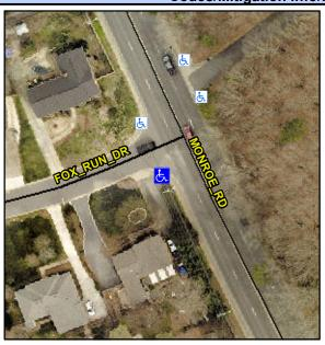
Street 1 Name Stop Condition-Street 2 Street 2 Name Stop Condition-Street 1 MONROE RD None **FOX RUN DR** StopSign Possible Solutions: Remove & Replace Curb Ramp With **Two New Directional Ramps or** Equivalent. Surveyor Notes: N/A PROW/ADA: Not Found, R304.2.2
