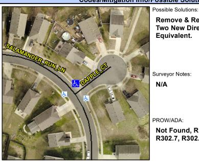
**SALAMANDER RUN LN** Street 1 Name Stop Condition-Street 1 Street 2 Name **DAPPLE CT** Stop Condition-Street 2 StopSign Remove & Replace Curb Ramp With **Two New Directional Ramps or** Equivalent.
