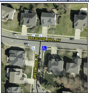
PRESCOTT HILL AV Street 1 Name Stop Condition-Street 2 None **GREYMORE CT** Street 2 Name Stop Condition-Street 1 StopSign Possible Solutions: Remove & Replace Curb Ramp With Two New Directional Ramps or Equivalent. Surveyor Notes: N/A PROW/ADA: Not Found, R304.5.1, R304.5.3
