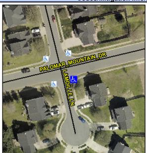
PALOMAR MOUNTAIN DR Street 1 Name Stop Condition-Street 2 None **LAMOILLE LN** Street 2 Name Stop Condition-Street 1 StopSign Possible Solutions: Remove & Replace Curb Ramp With Two New Directional Ramps or Equivalent. Surveyor Notes: N/A PROW/ADA: R304.5.1
