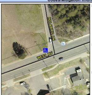
Street 1 Name **HOLABIRD LN** Stop Condition-Street 1 StopSign Street 2 Name N/A Stop Condition-Street 2 N/A Possible Solutions: Remove & Replace Entire Ramp. Surveyor Notes: N/A PROW/ADA: R304.5.1, R304.2.2, R304.5.3
