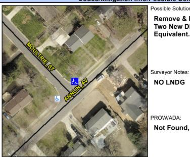
Street 1 Name Stop Condition-Street 1 Street 2 Name Stop Condition-Street 2 **MOULTRIE ST** StopSign **ANNLIN AV** None Possible Solutions: Remove & Replace Curb Ramp With **Two New Directional Ramps or** Equivalent.
