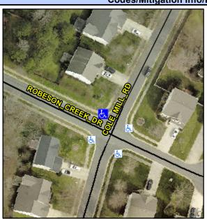
Street 1 Name Stop Condition-Street 2 Street 2 Name Stop Condition-Street 1 ROBESON CREEK DR None **COLE MILL RD** StopSign Possible Solutions: Remove & Replace Curb Ramp With Two New Directional Ramps or Equivalent. Surveyor Notes: N/A PROW/ADA: Not Found, R304.5.3
