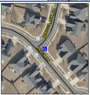
Street 1 Name Stop Condition-Street 2 Street 2 Name Stop Condition-Street 1 **REBECCA RUN DR** StopSign **BROCK RN** None Possible Solutions: Remove & Replace Curb Ramp With Two New Directional Ramps or Equivalent. Surveyor Notes: N/A PROW/ADA: Not Found, R304.5.1, R304.2.2, R304.5.3
