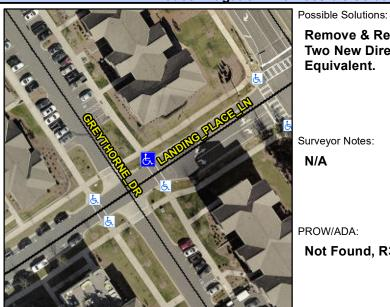
**LANDING PLACE LN** Street 1 Name Stop Condition-Street 1 None Street 2 Name N/A Stop Condition-Street 2 N/A Remove & Replace Curb Ramp With Two New Directional Ramps or Equivalent.
