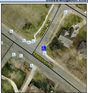
SHASTA LN Street 1 Name Stop Condition-Street 2 StopSign Street 2 Name N/A Stop Condition-Street 1 N/A Possible Solutions: Remove & Replace Entire Ramp. Remove & Replace Gutter. Surveyor Notes: N/A PROW/ADA: Not Found, R304.2.1, R304.2.2-Perp, R304.3.2-Para, R304.5.3, R304.5.4
