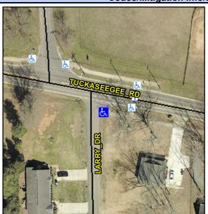
**TUCKASEEGEE RD** Street 1 Name Stop Condition-Street 1 None N/A Street 2 Name Stop Condition-Street 2 N/A Possible Solutions: Remove & Replace Detectable Warning System. Grind Gutter Lip. Surveyor Notes: NO CURB. DWS OS MEASURED TO **ASP** PROW/ADA: R305.1.4, R305.2, R302.7.2
