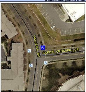
**GALLERIA BV** Street 1 Name Stop Condition-Street 2 **SARDIS CROSSING DR** Street 2 Name Stop Condition-Street 1 StopSign Possible Solutions: **Remove & Replace Curb Ramp With** Two New Directional Ramps or Equivalent. Surveyor Notes: N/A PROW/ADA: Not Found, R304.5.1, R304.2.2, R304.5.3
