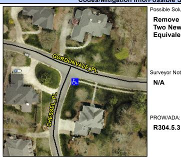
**GORDONVALE PL** Street 1 Name Stop Condition-Street 2 Street 2 Name **CHESSEL PL** Stop Condition-Street 1 StopSign Possible Solutions: Remove & Replace Curb Ramp With **Two New Directional Ramps or** Equivalent. Surveyor Notes: N/A
