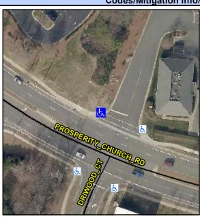
PROSPERITY CHURC Street 1 Name Stop Condition-Street 2 Street 2 Name DRIWO Stop Condition-Street 1 Sto Remove & Replace Curb Ramp With **Two New Directional Ramps or** Equivalent.
