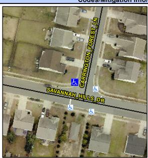
SAVANNAH HILLS DR Street 1 Name Stop Condition-Street 2 None **CARRINGTON FOREST LN** Street 2 Name Stop Condition-Street 1 StopSign Possible Solutions: Remove & Replace Curb Ramp With Two New Directional Ramps or Equivalent. Surveyor Notes: N/A PROW/ADA: Not Found, R304.5.1
